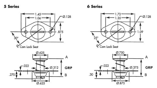
When you measure a spring (H), it is from the tab / Weldplate to the actual fastened point of the spring (B).
