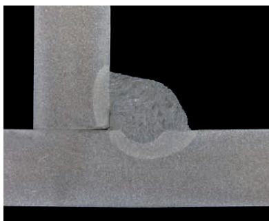
Figure 126. Lack of fusion.
