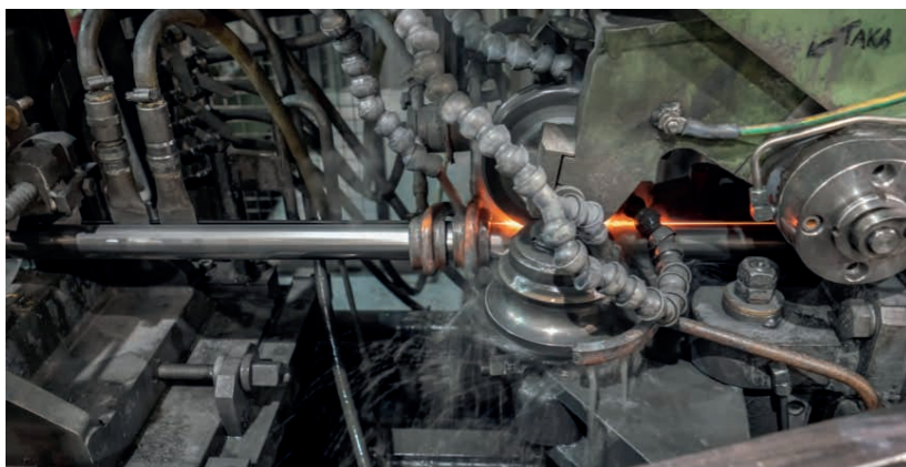
Figure 22. High frequency welding with induction coil, molten strip edges and squeezing between welding rolls.
