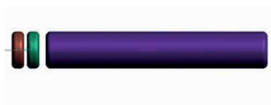
Figure 114. The mandrel in accordance with the recommendation in the Mandrel chart, whereby a tube to be bent at a slenderness of D/T=30 , requires a mandrel plus 2 balls to prevent wrinkling.
