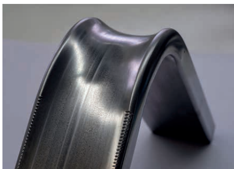
Figure 93. Tube bending defect: excessive flattening due to high D/T-ratio and bending without mandrel.
