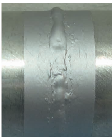
Figure 140. ARC-brazed joint of zinc-coated tube before salt spray test (left) and after salt spray test (right) with zinc spray protection.
