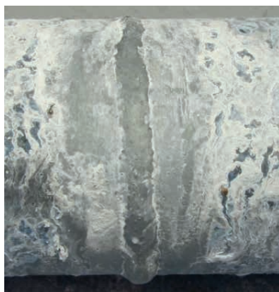
Figure 139. MAG-welded joint of zinc-coated tube after salt spray test without (left) and with zinc spray protection (right).
