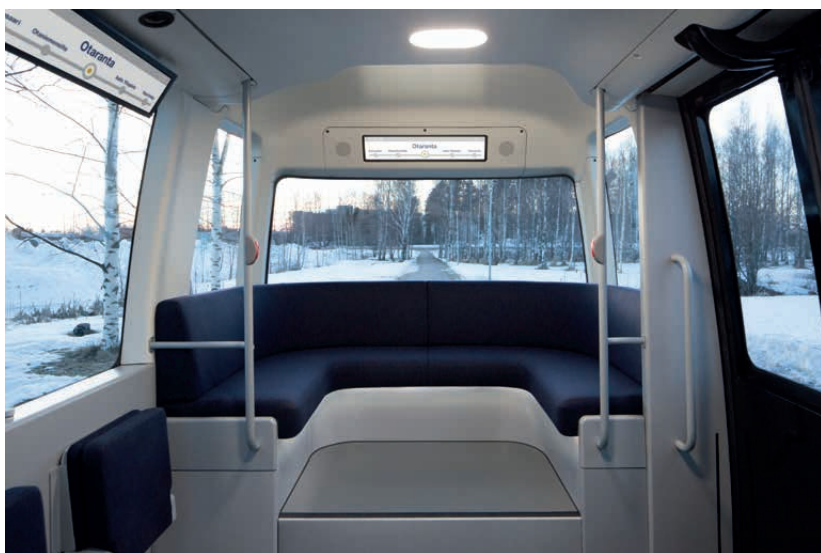
Figure 49. Autonomous vehicle, 10 seats, 6 standing places, Electric Gacha shuttle bus with frame manufactured from Docol Tubes. Photo: Justus Hirvi/Bonzu & Muji.
