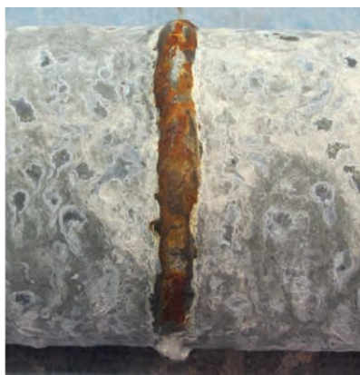
Figure 139. MAG-welded joint of zinc-coated tube after salt spray test without (left) and with zinc spray protection (right).
