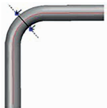
Figure 116a. Result of cross-section of stability indicating that the tube is still perfectly circular thanks to the mandrel used.
