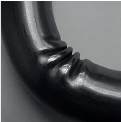
Figure 94. Tube bending defect: wrinkling due to extreme compression on inner radius.
