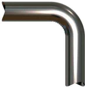
Figure 87. Wrinkles throughout bend area with wiper and mandrel in known position.
