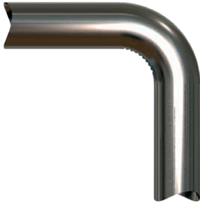
Figure 89. Heavy wrinkles through bend area only and linear scratches in grip area indicating clamp slippage.
