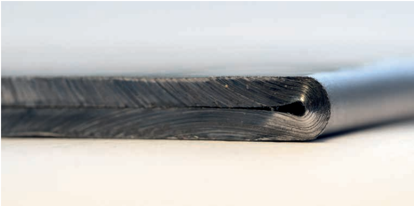
Figure 182. Example of the geometry of a straight, fully flattened tube. Note the gap next to the crimp despite extreme pressing force. The tube material is SSAB Form Tube 220 C.
