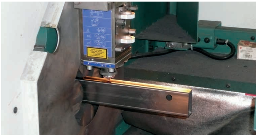
Figure 160. Centred tube by cutting head sensor. A separate measuring probe can also be used for centring.
