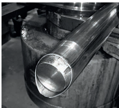
Figure 92. Tube bending defect: insufficient lubrication and therefore breakage.
