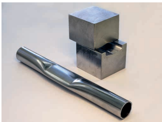
Figure 184. Round tube pressed with V-shaped tooling ending with smooth surface.
