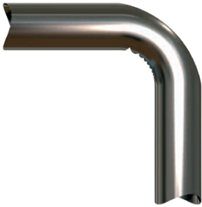
Figure 85. Excessive collapse with or without wrinkling throughout entire bend.
