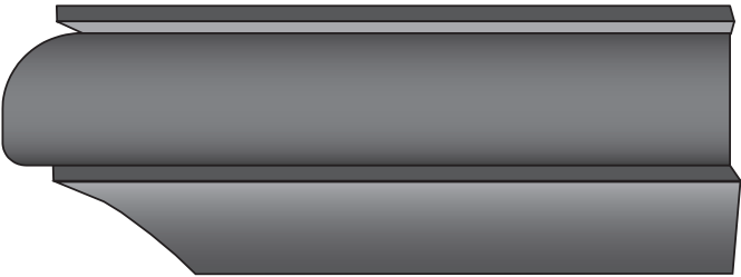
Figure 71. Wiper die usually made of softer material than the tube, e.g. aluminium-bronze.
