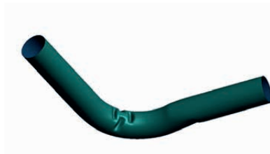
Figure 115b. The bend will collapse without mandrel.
