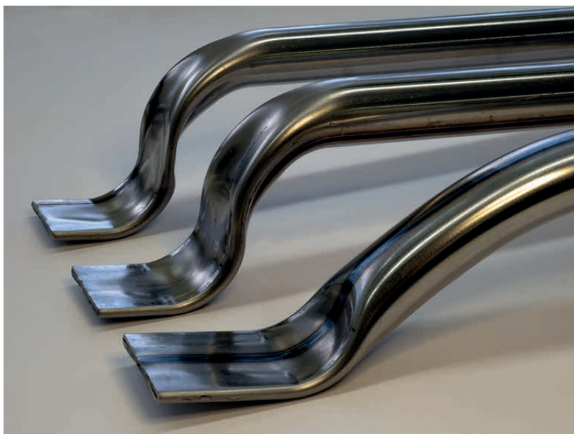
Figure 181. Flattened tube end. In connection with flattening, the end can be cut and/or punched.
