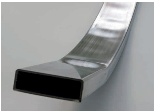
Figure 64. A risk for tube collapsing without internal support in roll bending.
