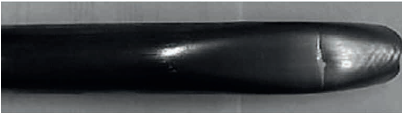
Figure 90. Tube bending defect: Mandrel seizing up with tube wall due to insufficient lubrication and wrong mandrel positioning and therefore breakage.
