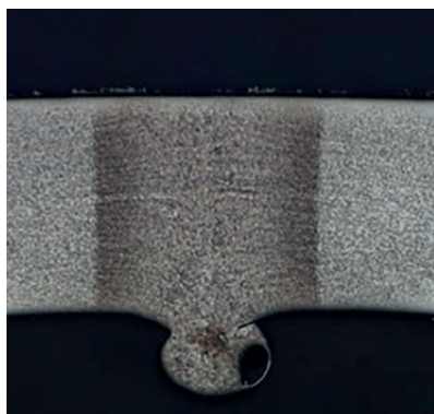
Figure 24. Example of a high-quality HF weld: The edges are at the same level, and the inside burr shows there has been enough welding energy and squeeze pressure to create a quality weld.
