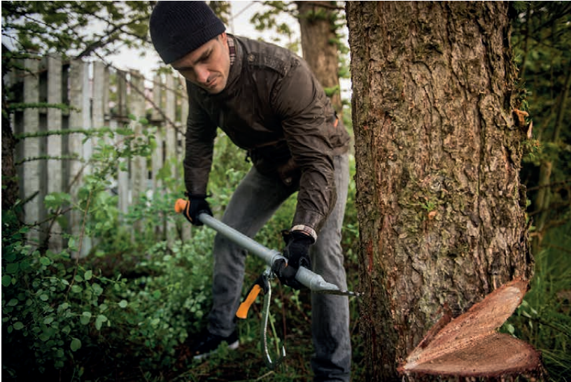
Figure 13. Felling lever with a tubular shaft of high-strength steel for wood logging. Courtesy of Fiskars.
