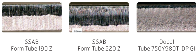
Figure 179. The effect of a change in shearing for steels of different strength levels. Punching parameters are the same for all materials for benchmarking purposes.
