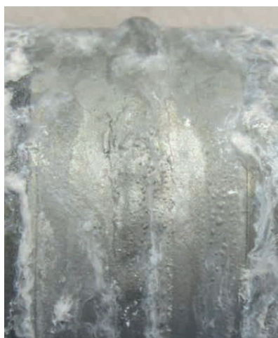
Figure 140. ARC-brazed joint of zinc-coated tube before salt spray test (left) and after salt spray test (right) with zinc spray protection.
