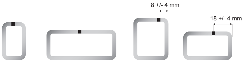
Figure 29. Possible weld seam positions and tolerances.
