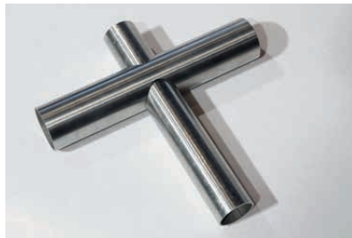
Figure 164. High precision tube joining in the form of through cutting.
