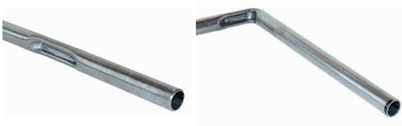
Figure 60. Decreasing bending radius by decreasing “D” of the tube.
