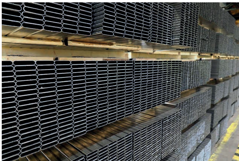
Figure 186. Light protection oil means light rust protection during transportation and storage, it is not intended for outdoor exposure.
