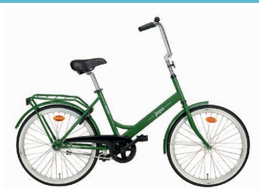
Figure 5. Bicycle frame, including flat oval SSAB Form Tube 220 C 60x30x2.0. Courtesy of Helkama Velox Oy.
