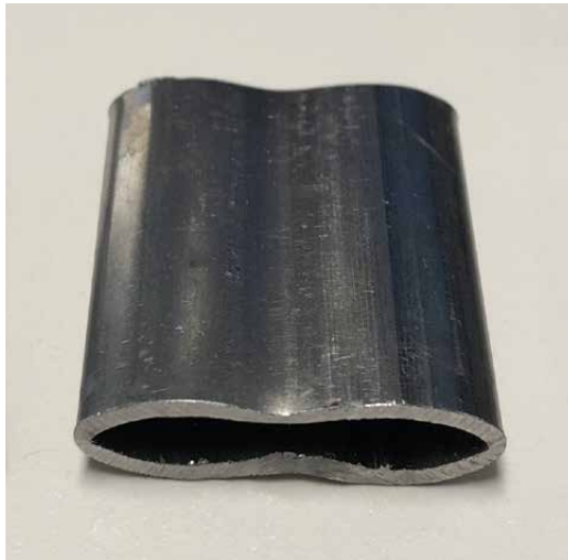
Figure 183. Round tube pressed with flat tooling ending with an undesirable infinity sign cross section.
