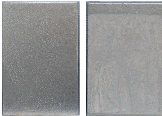
Figure 155. 24h in QCT 60°C. Left picture is Z600 and right one is hot dip galvanised.
