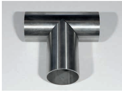
Figure 163. High precision tube joining “edge-to-edge” with curved surfaces.
