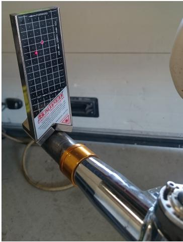
Figure 18: Sniper mounted on spindle. See the two red dots on the panel, the most left dot comes from the other end and indicates the camber as well as the toe setting.
