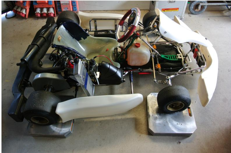
Figure 19: Kart set up for measuring cross weight.
