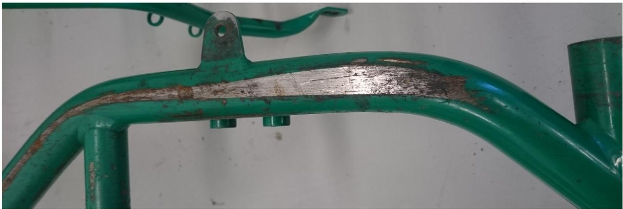
Figure 6: Grinding wear on the underside of the main chassis tubes.
